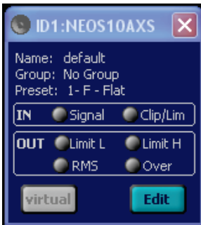
Fig.20 Example of an active loudspeaker control panel.
