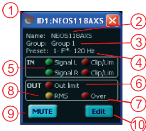
Fig.38 Subwoofer's control panel.
