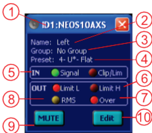
Fig.37 Satellite loudspeaker's control panel.
