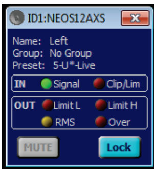
Fig.111 Control panel for a LOCKED loudspeaker.
